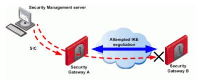
To configure a VPN between Security Gateways A and B through SmartConsole, the administrator must install a Policy from the Security Management Server to the Security Gateways.
