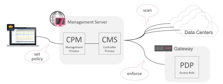
Here's how it works: the CloudGuard Controller scanner periodically polls objects in the data center. The scanner then connects to the management CPM process to update the data center objects and it also connects to the PDP process on the gateways to update the data center objects used in the gateway security policy (<u>sk115657</u>).
