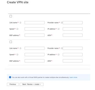
IP Address= Public IP address of the on-premises firewall using this link. Optionally, you can provide the private IP address of your on-premises VPN device that is behind ExpressRoute. If you add multiple Links you can't use the same Public IP address for different links into the same VPN configuration.
